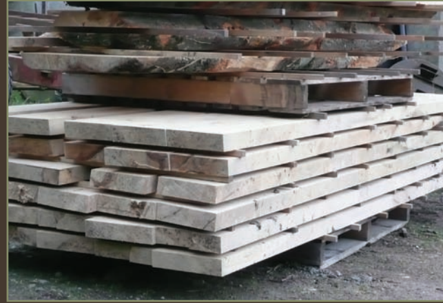
Sawn Timber prepared for Air Drying.
