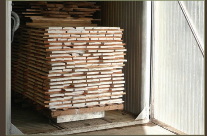
Kiln Drying the timber stack.
